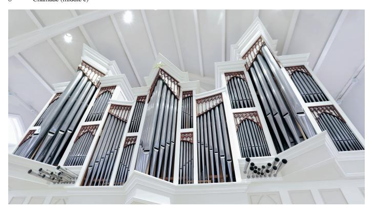
Kellner 1/5-comma well temperament Detached Console Wind system with one wedge-shaped bellows fed by a silent blower Suspended key-action, self-compensating for seasonal changes Electric stop action with solid-state combination action Compass: Manuals, C-a"'; Pedal, C-f'
